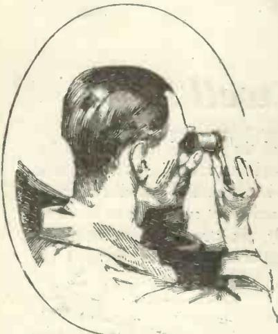
Illustration showing laboratory worker taking a temperature reading by means of the Pyrometer—an instrument for measuring temperatures which cannot be obtained by means of the ordinary thermometer system.
